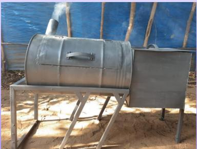
The idea generated by BVoc Fish Processing Technology students was developed through MESAC, IEDC. The working model was used to smoke fish in a controlled atmosphere. This regulated the phenolic content taken up by the fish fillets.
